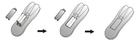
Figure 15 Battery replacement process
